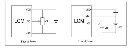
$V_{DD-}V_0$ : LCD Driving voltage VR: 10k~20k
