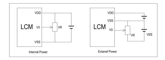
V<sub>DD~</sub>V<sub>0</sub>: LCD Driving voltage
