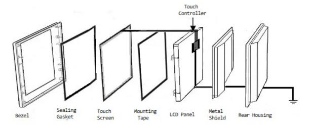
Some common applications for capacitive touch panels include cellphones, navigation systems, tablets, cameras, and computer screens. Capacitive touch panels can be incorporated into any TFT or other custom display applications, and has the added benefit of durability as well as flexibility.
