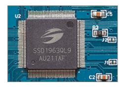
This controller would be a good choice for a display of this resolution, color depth and communication interface. This would support an AVR if the 8-bit MCU communication interface is chosen. If a faster interface, such as the 16/18/24-bit MCU interface, is used to communicate with this controller, the AVR would be insufficient. An ARM microcontroller is often a better option to consider even with the addition of a graphics controlling chip.
