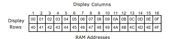
For display communication, the data is sent to registers in RAM to define display parameters where the data is transferred automatically. The control byte is made up of the register command and the continuation bit. The defines whether the control byte is represented as a command or data.
