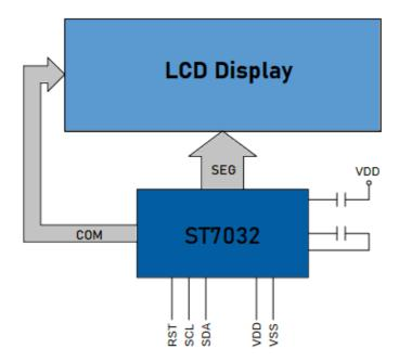
The I2C interface would not be capable of refreshing an image on a TFT display. TFT displays typically have a higher resolution with each pixel containing color data. This interface would not communicate fast enough to update the display with the desired response. However, the I2C interface can be used for TFT initialization commands.
