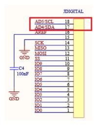
Below is the pinout of the display with the I2C pins and their description.
