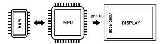
The video mode of the MIPI DSI protocol relies on internal RAM to be provided by the host processor. It is used when the display does not provide internal display RAM or if the display does not have an internal controller. The synchronization event can be sent in brief low power operation events or as null data events. These events also structure the begin and end of a DSI data packet.
