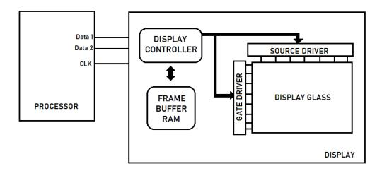
Another benefit of using internal display RAM is that the physical memory addresses correspond to the pixel display area. In other words, the frame buffer is the same size as the resolution. The internal display RAM provides the exact amount of memory for the display resolution. This makes reading and writing to RAM simple. Display RAM typically provides enough memory for one full page of image data at high color. This can often be more than what is provided on the MPU.
