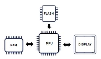
High resolution displays have a larger number of pixels and require more memory. An increased color depth means there is more data assigned to each pixel. For true color (RGB-888) each pixel is assigned 24-bits of color. This data needs to be stored in a location accessible by the microprocessor and the display. The minimum memory requirement for the framebuffer is calculated by the following equation.
