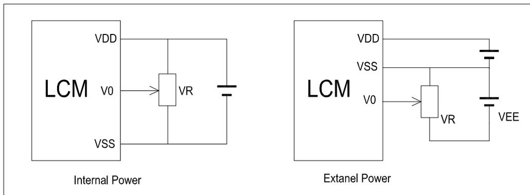
$V_{DD}-V_0$ : LCD Driving voltage
