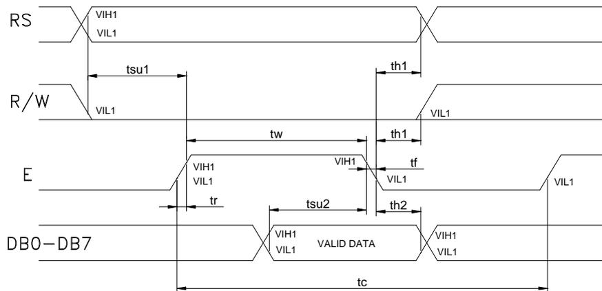
Read cycle ( $T_a=25^\circ\text{C}$ ,  $V_{DD}=3.3\text{V}$ )
