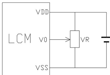
V<sub>DD</sub>-V<sub>0</sub>: LCD Driving voltage
