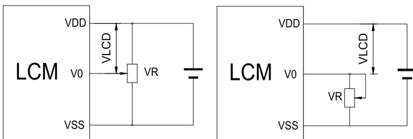
V<sub>DD</sub>-V<sub>0</sub>: LCD Driving voltage
