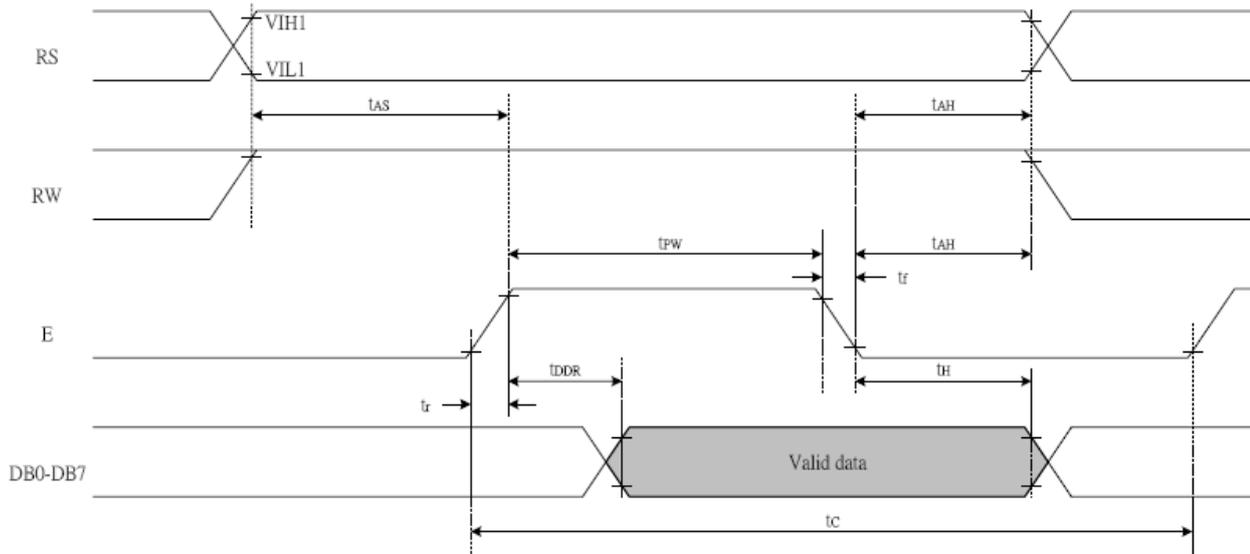
**Write cycle (Ta=25°C, VDD=5.0V)**
