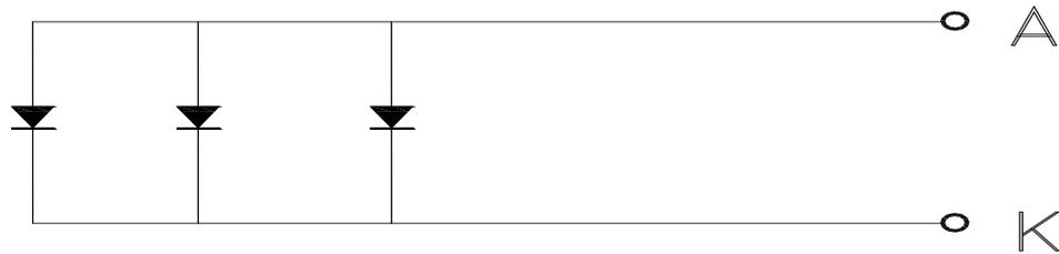
LED CIRCUIT DIAGAM(LED 1X3=3 dies)
