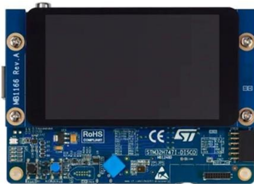
Figure 3: STM32H747I-Disco Development Board
