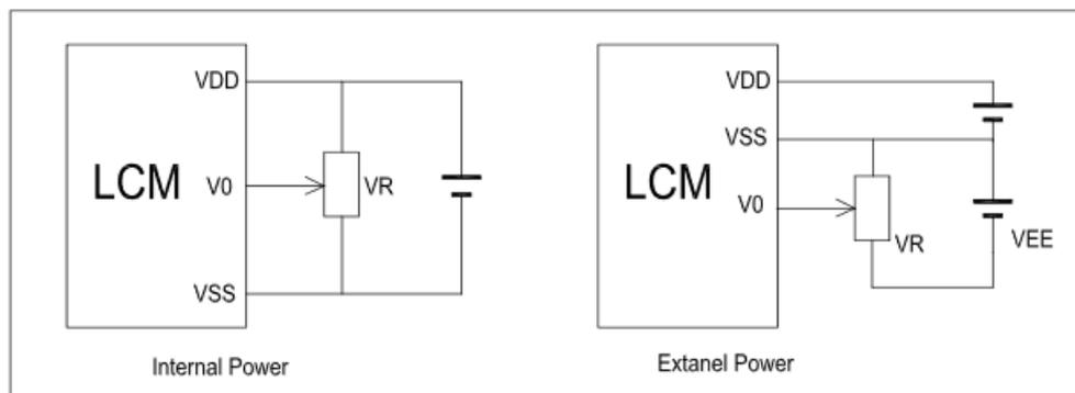
VDD-V0: LCD Driving Voltage
