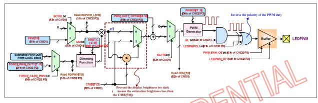
Internal Display Backlight Control Combined With CABC and Manual brightness adjustment
