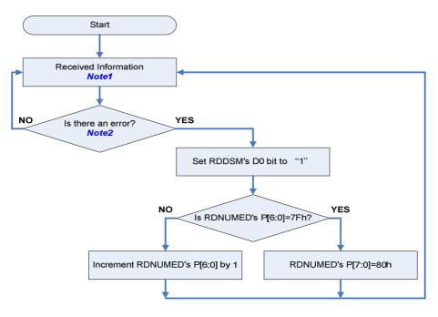
Note1: This information can be interface or packet level communication but it is always from the MCU to the display module in this case.
