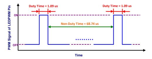
The same, when PWM frequency is 14.32 KHz, and PWM duty of LEDPWM is 256 (Reading the register "RDDISBV[7 : 0]" = FFh), then the duty time can be estimated as shown in below :
