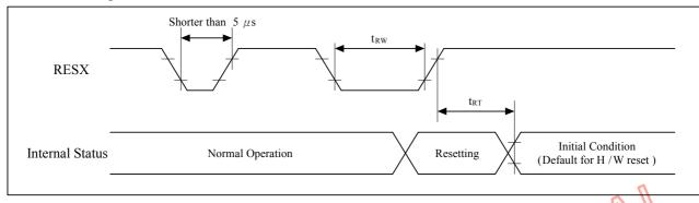
Figure 7.3.4 Reset Operation
