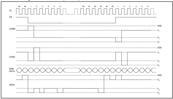
Two-frame alternating current drive-wave form (SPLC501C)
