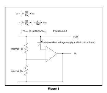
$V_{REG}$  is the IC-internal fixed voltage supply, and its voltage at  $T_A$  =  $25^\circ\!\mathbb{C}$  is as shown in Table 9.
