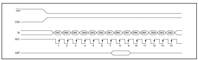
Figure 1: serial interface signal chart.
