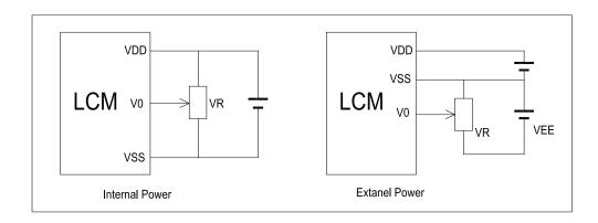
$V_{DD\sim}V_0$ : LCD Driving voltage
