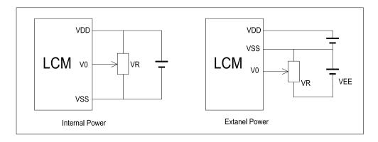
$V_{DD-}V_0$ : LCD Driving voltage VR: 10k~20k
