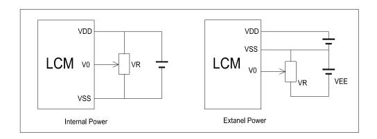
$V_{DD\sim}V_0$ : LCD Driving voltage VR:  $10k\sim20k$
