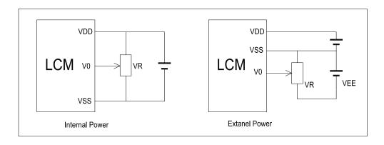
V<sub>DD~</sub>V<sub>0</sub>: LCD Driving voltage VR: 10k~20k
