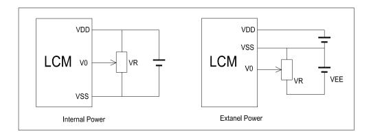
V<sub>DD~</sub>V<sub>0</sub>: LCD Driving voltage
