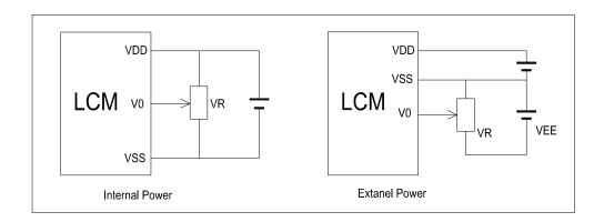
$V_{DD^{\sim}}V_0\text{: LCD Driving voltage}$
