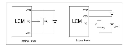
V<sub>DD~</sub>V<sub>0</sub>: LCD Driving voltage
