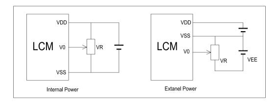
V<sub>DD∼</sub>V₀: LCD Driving voltage
