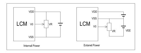
VDD~V0: LCD Driving voltage VR: 10k~20k
