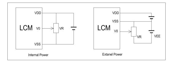
$V_{\text{DD-}}V_0$ : LCD Driving voltage
