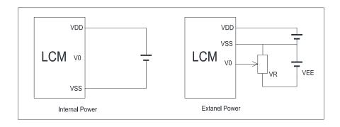
$V_{\text{DD}\text{-}}V_0\text{: LCD}$  Driving voltage
