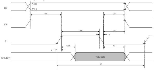
Write cycle (Ta=25°C, VDD=5.0V)
