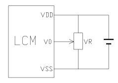
VDD~V0: LCD Driving voltage
