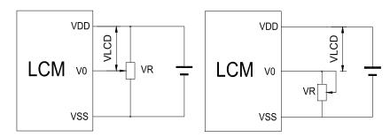
VDD~V0: LCD Driving voltage
