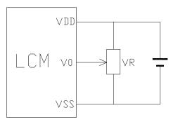
V<sub>DD-</sub>V<sub>0</sub>: LCD Driving voltage VR: 10k~20k
