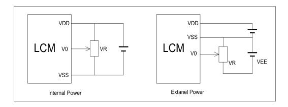
V<sub>DD~</sub>V<sub>0</sub>: LCD Driving voltage
