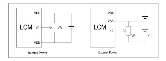
V<sub>DD~</sub>V<sub>0</sub>: LCD Driving voltage
