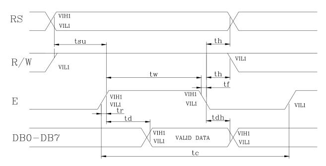
Write cycle (Ta= $25^{\circ}$ C, V<sub>DD</sub>=5.0V)
