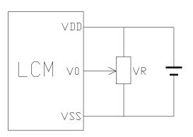
V<sub>DD~</sub>V<sub>0</sub>: LCD Driving voltage VR: 10k~20k
