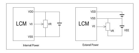
VDD~V0: LCD Driving voltage VR: 10k~20k
