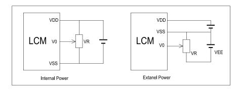
VDD~V0: LCD Driving voltage VR: 10k~20k
