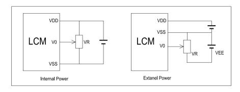
VDD~V0: LCD Driving voltage VR: 10k~20k
