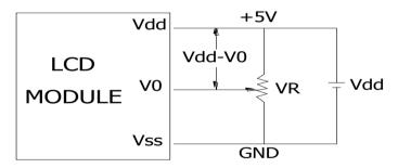
Vdd-V0: LCD Driving Voltage VR: 10K - 20K
