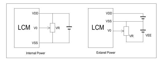
$V_{DD\sim}V_0$ : LCD Driving voltage
