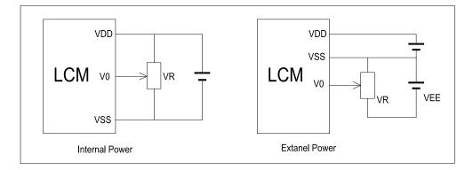
$V_{DD-}V_0$ : LCD Driving voltage VR: 10k~20k
