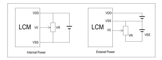
$V_{DD\sim}V_0$ : LCD Driving voltage
