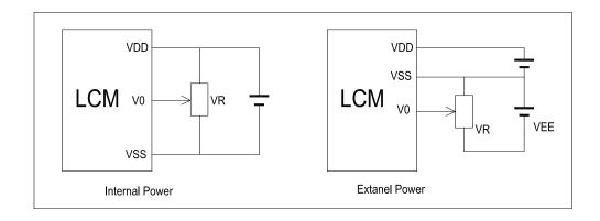
V<sub>DD~</sub>V<sub>0</sub>: LCD Driving voltage
