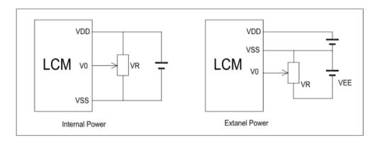
VDD-V0: LCD Driving Voltage VR: 10k-20k
