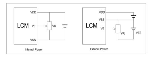
VDD-V0: LCD Driving Voltage VR: 10k-20k
