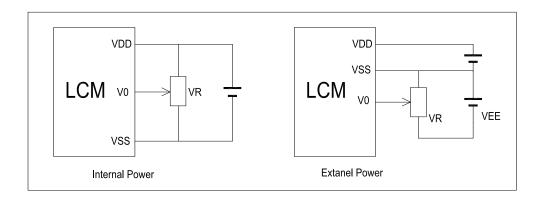
V<sub>DD~</sub>V<sub>0</sub>: LCD Driving voltage
