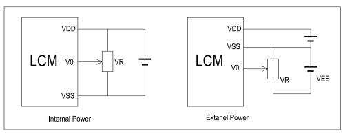
$V_{DD-}V_0$ : LCD Driving voltage VR: 10k~20k
