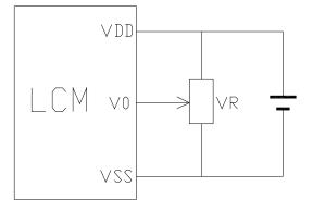
V<sub>DD-</sub>V<sub>0</sub>: LCD Driving voltage VR: 10k~20k
