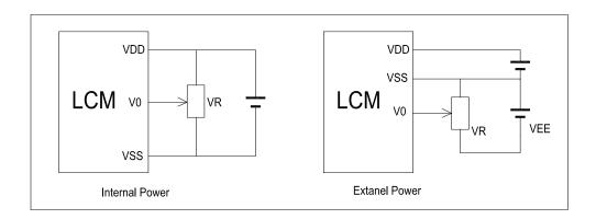
$V_{\text{DD}\text{-}}V_0\text{: LCD}$  Driving voltage
