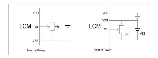
$V_{DD^{\sim}}V_0$ : LCD Driving voltage
