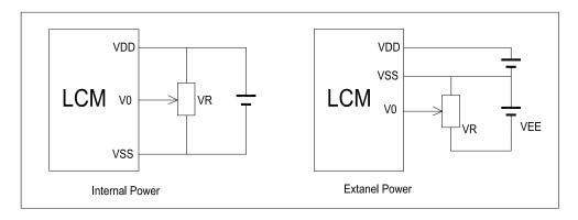
V<sub>DD~</sub>V<sub>0</sub>: LCD Driving voltage VR: 10k~20k
