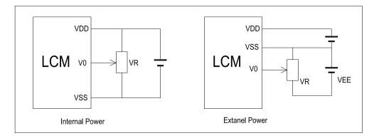
V<sub>DD-</sub>V<sub>0</sub>: LCD Driving voltage VR: 10k~20k
