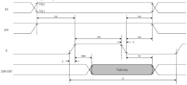
**Write cycle** (Ta=25°C, VDD=2.7V)
