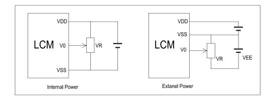
$V_{DD^{\sim}}V_0\text{: LCD Driving voltage}$
